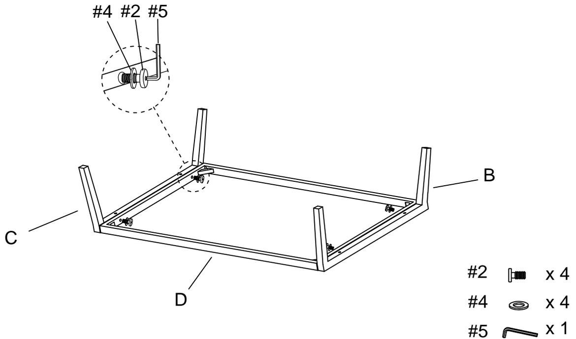
Step 2: Attach left leg (part B) and right leg (part C) to seat panel (part A) using long bolts (part #3), flat washers (part #4) and allen wrench (part #5).
