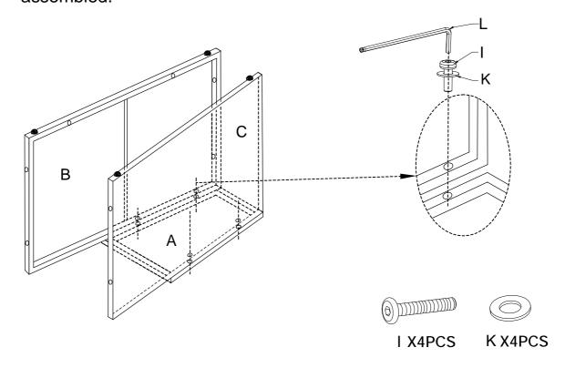
**Step 2**. Attach Front Panel(D) to assembled parts(A,B&C) using Long Bolts(I), Washers(K) and Allen Key (L).
