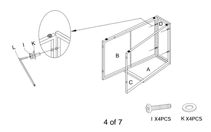
**Step 3**. Attach Back Panel(E) to assembled parts(A,B,C&D) using Long Bolts(I), Washers(K) and Allen Key (L).
