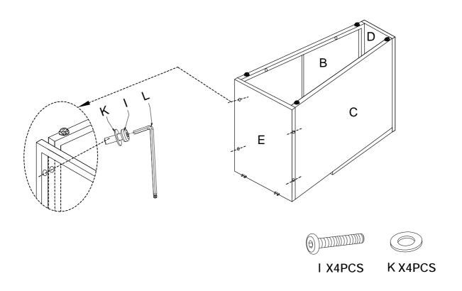
**Step 4**. Attach Bottom Panel(F) to assembled parts(A,B,C,D&E) using Long Bolts(I), Washers(K) and Allen Key (L).
