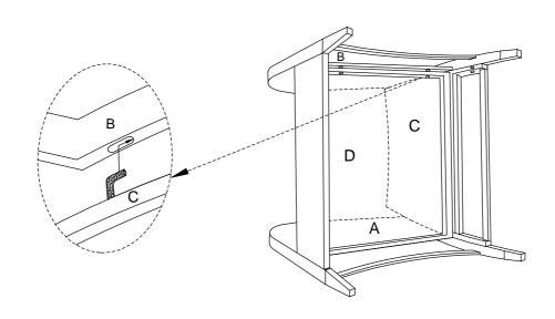
**Step 5**. Attach Right Arm Panel (B) to assembled parts(A,C&D) using the Short Bolts (G),Long Bolts (H),Washers (J),Nuts (I), Wrench (K), and Allen Key (L).
