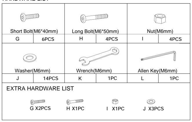
**Step 1**. Lay Left Arm Panel (A) down on a flat surface. Attach Seat Panel(D) to Left Arm Panel(A) using the Short Bolts(G),Long Bolts(H), Washers(J),Nuts(I), Wrench(K) & Allen Key (L). NOTE: Please do not fully tighten bolts until unit is fully
