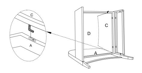
**Step 3**. Attach Back Panel(C) to Left Arm Panel(A) and Seat Panel (D) using the Short Bolts(G) Washers(J) & Allen Key (L).
