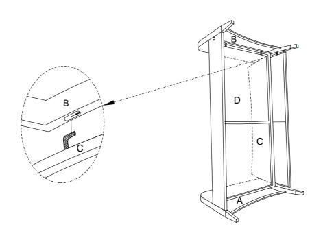
**Step 5**. Attach Right Arm Panel (B) to assembled parts(A,C&D) using the Short Bolts (G),Long Bolts (H),Washers (J),Nuts (I),Wrench (K), and Allen Key (L).
