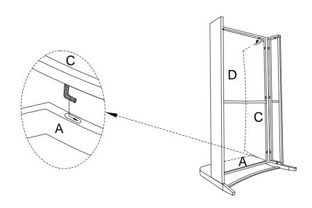
**Step 3**. Attach Back Panel(C) to Left Arm Panel(A) and Seat Panel (D) using the Short Bolts(G) Washers(J) & Allen Key (L).
