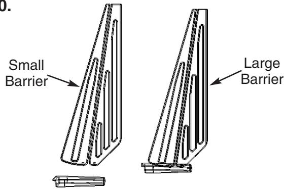
Snap Small and Large Barrier Sections into slots on Lower Base as shown.
