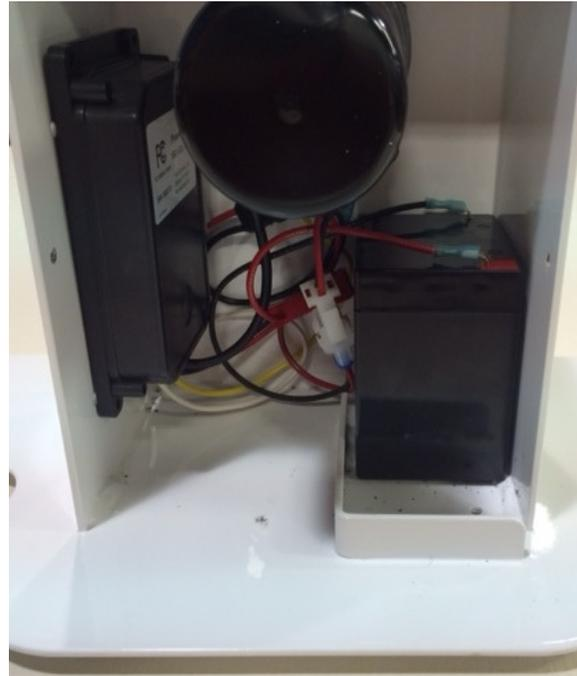
Properly installed battery
