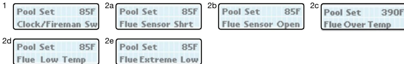
1. Fireman's Switch - When used with mechanical time clock, a Fireman's switch turns the heater OFF about 15 minutes before the pump is turned off. This is a function of the switch, not the circuit. Recommended for single speed pumps. Circuit can also be used as heater enable/disable signal, when needed.
