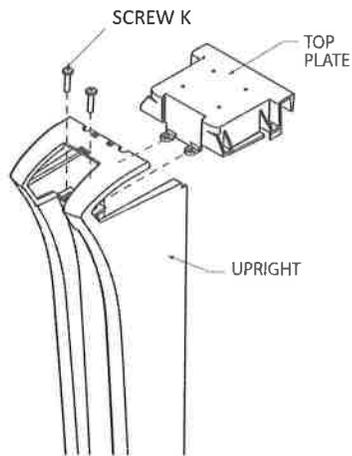
Install the joiner plates on top of each upright then install metal screws at the top of the support posts, making sure the support posts are perpendicular to the ground.
