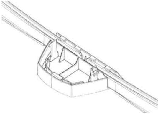
Assemble all bottom tracks to the bottom plates to form a perfect circle with a diameter and a radius in accordance to the chart
