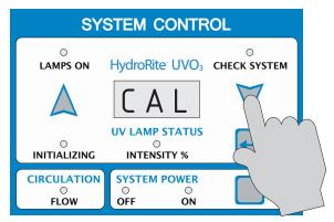
3) Push the arrow keys until "CAL" is shown in the display.
