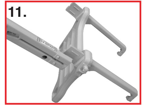
11. Overlap the flat end of the ladder leg onto the flat end of the handrail. Insert one of the 1/4 - 20 x 1" bolt through the ladder leg into the handrail. Place one of the 1/4 - 20 hex nuts into the recessed area on the handrail and tighten using a Phillips screwdriver. Install the second nut and bolt.
