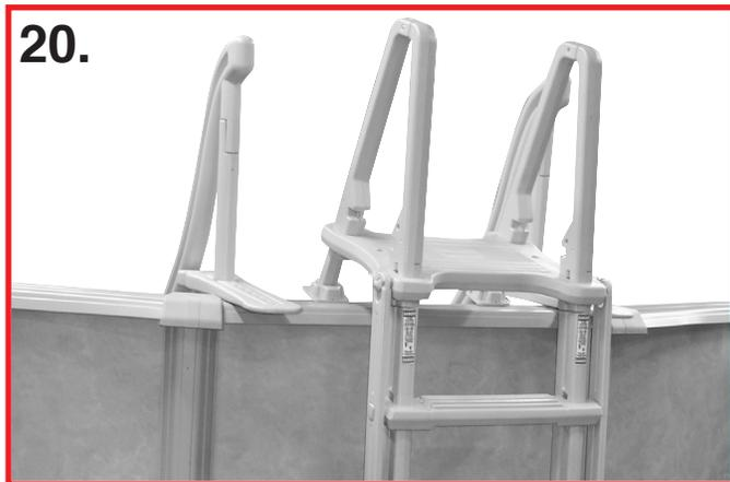
With the step in location place your 8100x ladder over the pool wall. Depending on the outside height of swimming pool ledge extension boots can be removed or slid up or down until the ladder platform is resting on top of the swimming pool top ledge. If necessary remove or add soil to raise or lower ladder. **The 8100x ladder platform must rest on top of the swimming pool ledge for support.**
