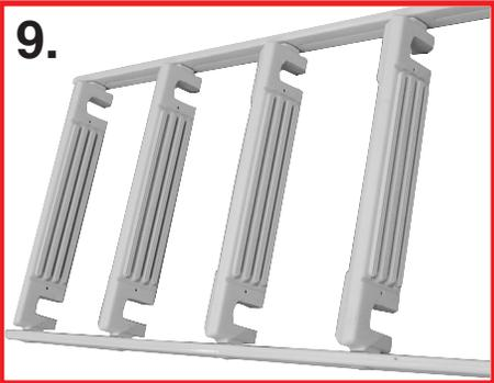
9. Separate the the swing up assembly from the ladder legs and set aside.
