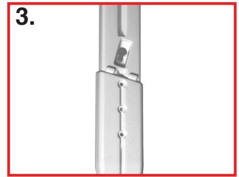
3. Slip the (2) two extension boots over the ends of the ladder legs. They will need to be all the way on if the outside dimension is 52" and backed off one hole if the outside dimension is 54".
