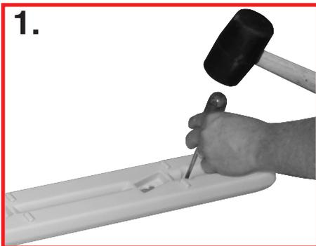
1. Place (2) two ladder legs on a flat surface. Using a Phillips screwdriver tap out the plastic film from the three holes on the bottom of each leg.
