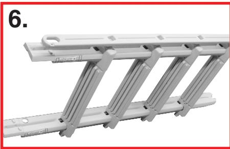
6. Stand the assembly up on edge and place the tread connector over the square ends on the (4) four treads. The large oval hole on the tread connector must be on the same end as the flat side on the ladder legs.
