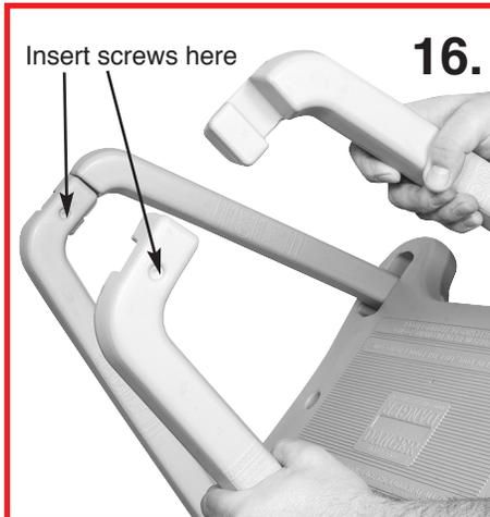
16. Using a #10 x 1-1/4" screw fasten the upper ends of the handrails together as shown. Repeat for opposite side.
