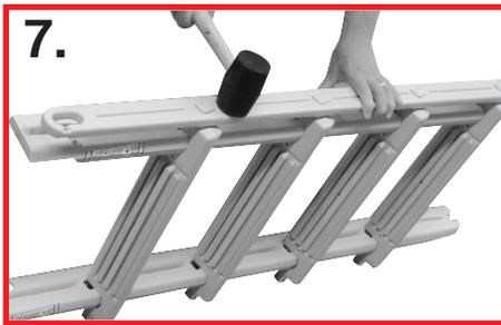
7. Using a rubber mallet tap the tread connector onto the square ends of the treads until they are firmly seated. A little liquid soap on the tread end will help.
