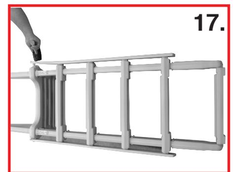
17. Flex the oval openings on the swing up assembly (from step #9) over the two round tabs on the platform. Using a rubber mallet tap down on the tread connector until seated over the round tab. **It may require several hard hits with a rubber mallet to get tread connector over round tabs.**
