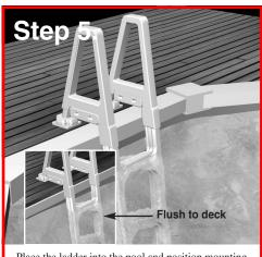
Place the ladder into the pool and position mounting blocks on deck. Slide the adjustable tubes up or down as needed until mounting blocks are sitting flush on the deck. Ladder MUST rest on pool bottom. If not, EB100 riser(s) are required. (See page 3 to order)
