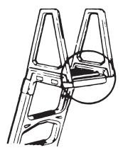
Platform provides extra "step" at top of ladder. Prevents swimmers from stepping on pool top.
