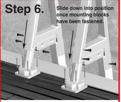
Drill four pilot holes (1/8") through holes in each block into wood surface. Fasten blocks to deck using the four #10 x 1-1/4" screws per mounting block. Drill three holes through each side of each handrail at the pre-marked locations. Fasten using three #10 x 1-1/4" screws.
