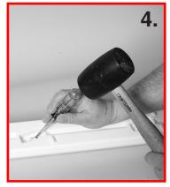
Using a Phillips screwdriver, knock out all four of the keyhole slot inserts from two of the ladder legs.
