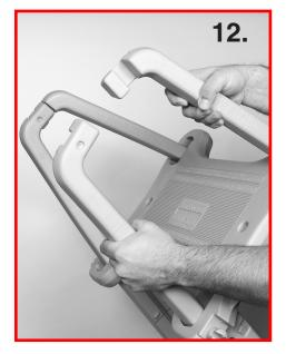
Tap the platform down until fully seated on the lugs as shown.
