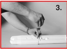
Using four 1/4-20 x 2" long bolts and four acorn nuts fasten the extension boots to the ladder legs
