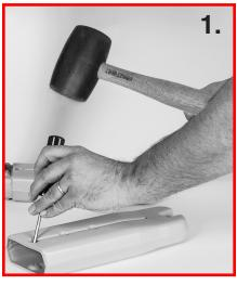
If the round plastic inserts, on the sides of the extension boots, are still in place, remove them with a phillips head screwdriver as shown.
