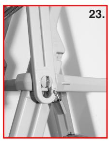
Swing up portion of ladder shown in "up" position, secured with padlock.
