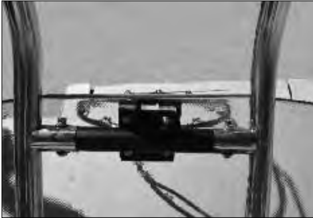
Fig. 24 Support Poles Over Crossbrace
