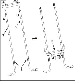
**IMPORTANT:** Ensure the J-shaped legs are pointing outwards before installing the steps.
