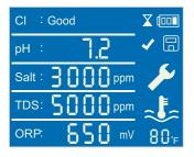
**Safedip** Measures Salt Content, pH, Free Chlorine DHP, TDS and Water Temperature
