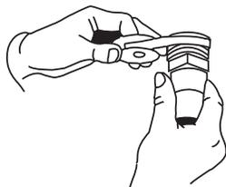
**5.** Screw adapter into the other side of POOL FROG Cyclers. Hand tighten. Finish tightening by turning 1 to 2 revolutions with a pipe wrench.
