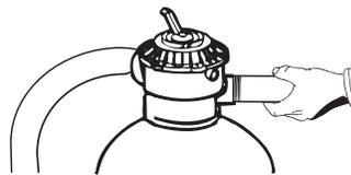
**3.** Screw either side of POOL FROG Cyclers on to open nipple end until upright and secure.
