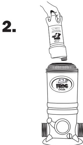
Insert upside down into the open center of the POOL FROG Mineral Reservoir pushing down firmly on FROG BAM bottle allowing key in POOL FROG Cyclor to puncture seal.
