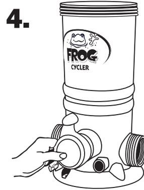
Carefully insert control dial back into housing.
