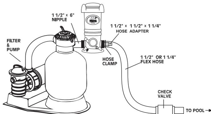
**7.** To prevent damage to heaters or filters, see your dealer about installing a **corrosion resistant check valve** which will reduce the back flow of chlorine gas when the Cyclers is turned off.
