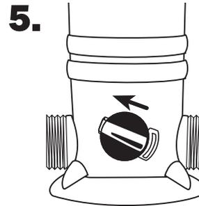
Replace locking pin by pushing it through the slots on the dial until it locks into place.
