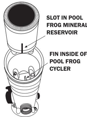
Find slot on side of POOL FROG Mineral Reservoir and line up with fin inside the POOL FROG Cyclor. Lower POOL FROG Mineral Reservoir into POOL FROG Cyclor until secure.
