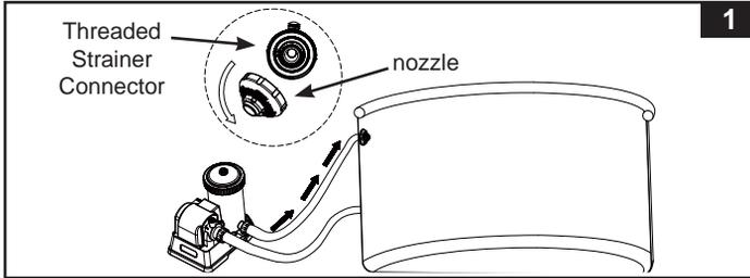
2. Screw the end of hose A (8) with adaptor to the threaded strainer connector, from inside of the pool. See Fig. 2.
