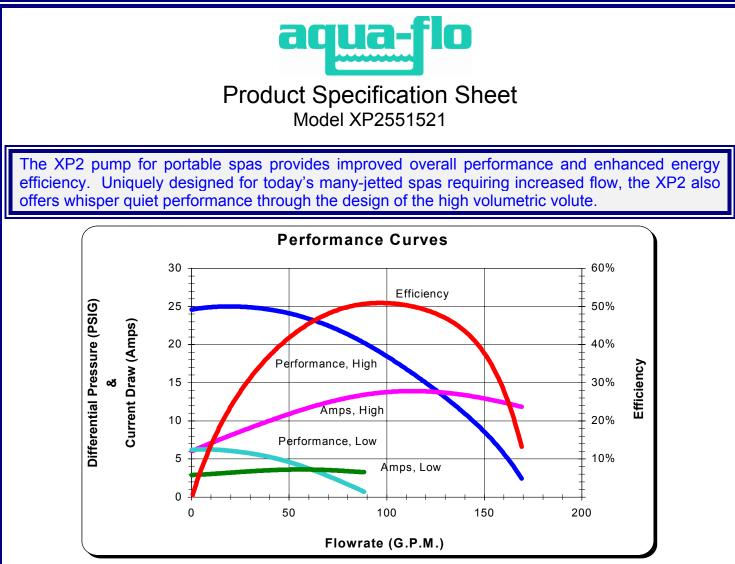
These performance curves are a result of in-lab testing using 3" suction line, actual performance may vary based on manufacturing tolerances and application.
